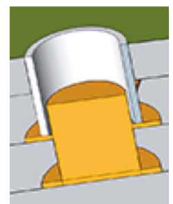
Figure 10: Insufficient back-drilling depth leaving a stub antenna
